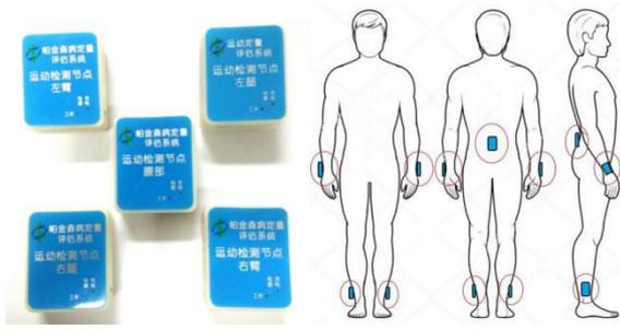
Figure 1. Wearable sensor nodes and the wearing positions.
