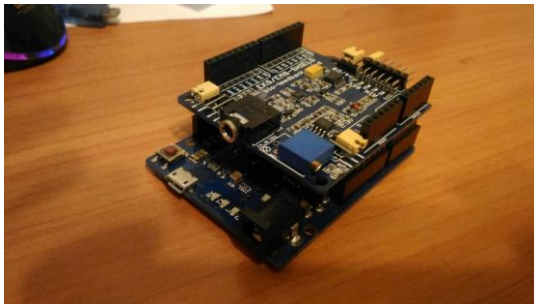
Fig. 2. Device for fixing EMG signal.
