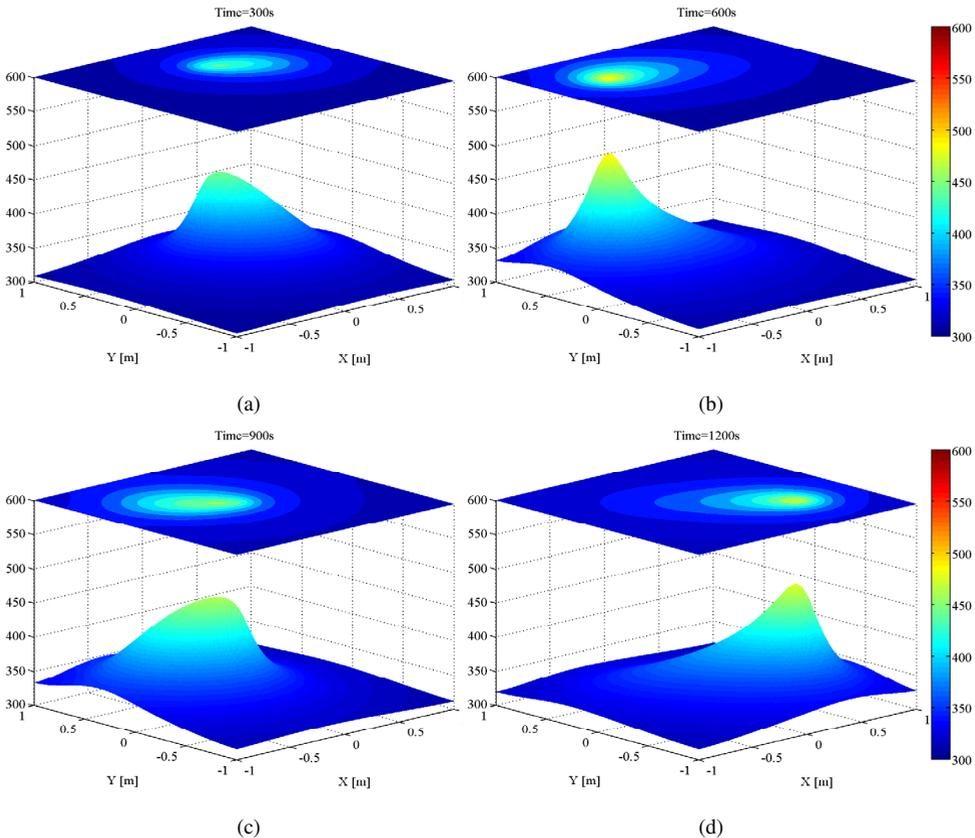
**Figure 1.** Spatial evolution of temperature on the plate generated by heat source
