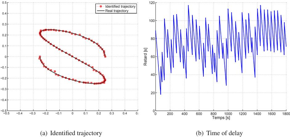
**Figure 3.** Results of identified trajectory and time of relay
