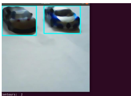
Figure 7. Car Detection by Contours
