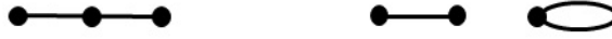
Figure 8 One connected and one disconnected graph with degree sequence \{T_1 = 1, T_2 = 1, T_3 = 2\}
