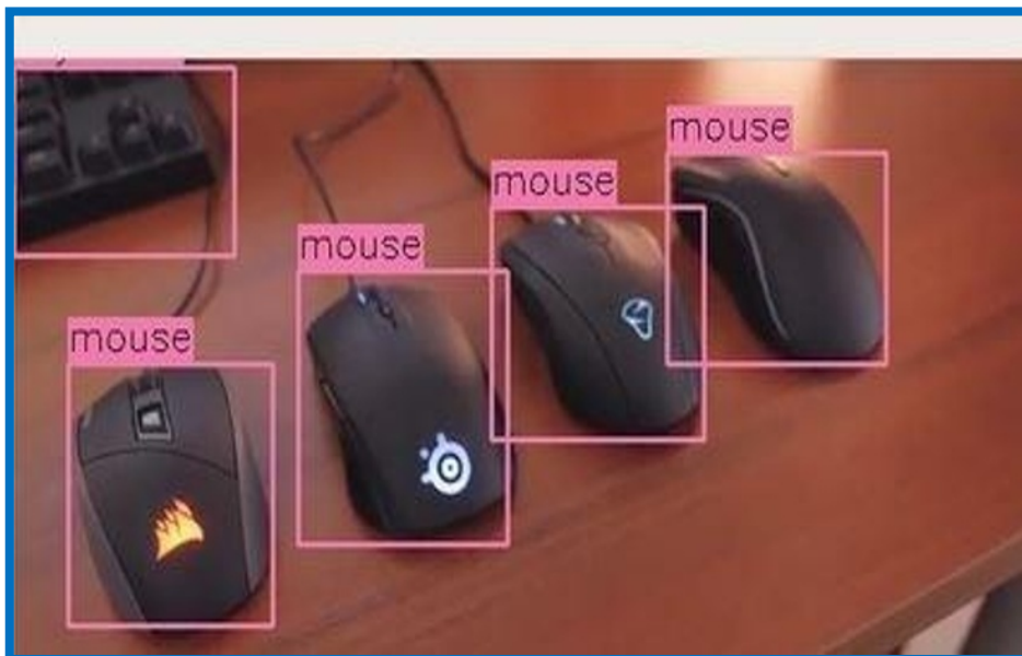
Fig. 4. Experimental verification of the neural network YOLO v3 - tiny on the Raspberry Pi 3B +.
