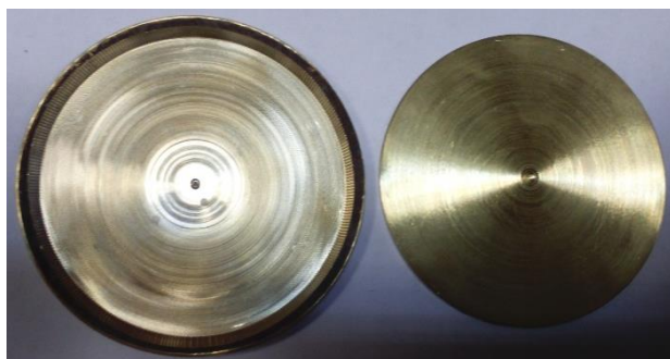
Fig. 4. Blank with a shoulder (left) and after processing without a shoulder (right).
