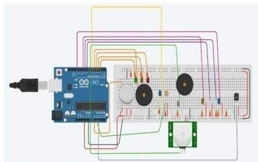
Fig 12: Sensor Module
