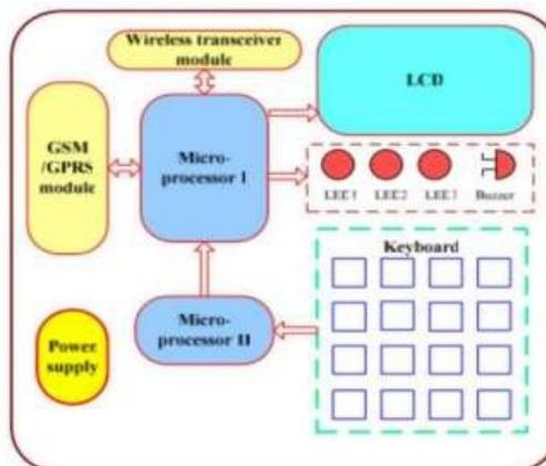
**Fig 1:** GSM/GPRS based wireless Home Security System[5]
