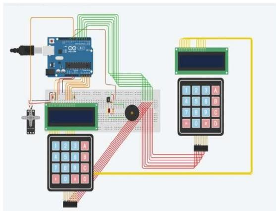
Fig 11: Password Validator Module
