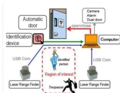
**Fig 2:** Human Tracking Method with Laser Range Finder[6]
