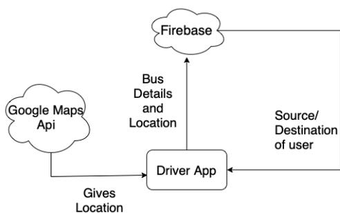
Figure 2: Functional Block Diagram of Driver Unit
