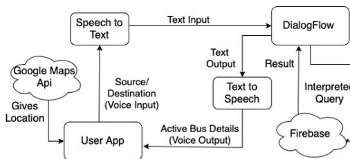
Figure 1: Functional Block Diagram of User Unit
