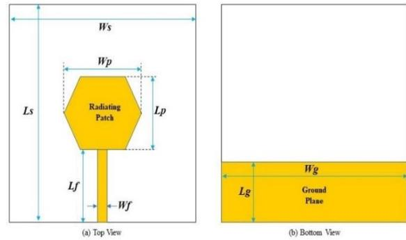
Fig. 3. Design details of dimensions of HMSA
