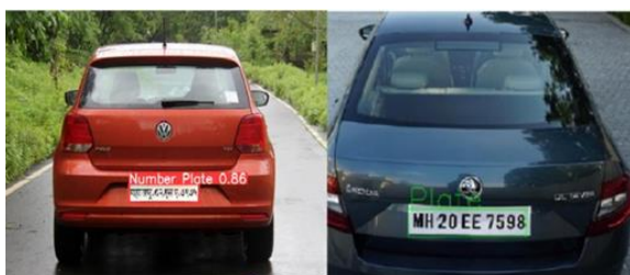
Fig. 4. Image after the detection of license plate using YOLOv5 Model
