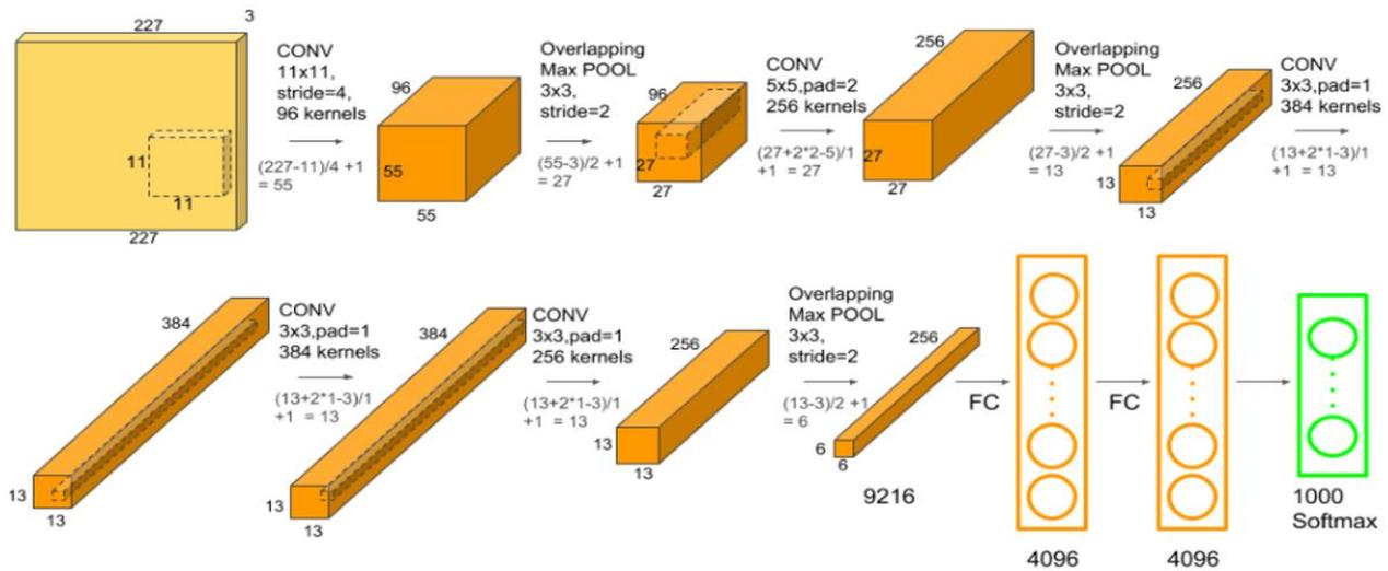
**Fig. 2.** AlexNet Architecture[10]. The figure depicts the architecture of AlexNet with its 5 convolution layers, 3 max-pooling layers and 3 fully connected layers.
