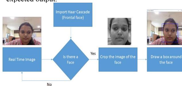
Figure 7: Face detection using Haar Features
