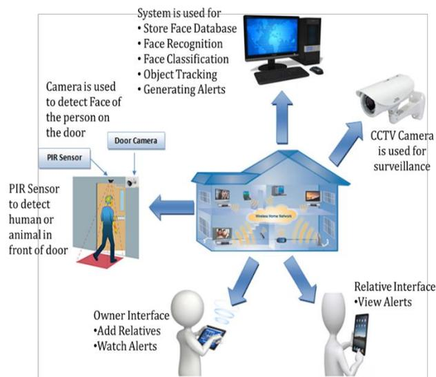
Figure 1: Home safety measures using face recognition and PIR.
