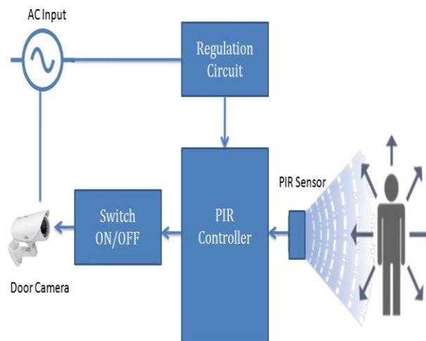
Figure 3: Passive Infrared (PIR) controller diagram
