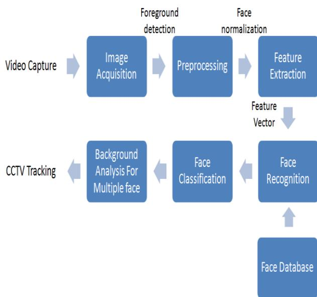
Figure 4: Flow chart of Face Recognition and Classification
