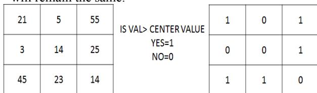
Figure 8: Local binary pattern histogram generating 8-bit number
