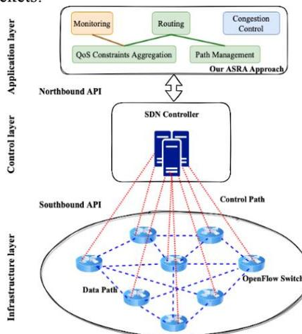
**Fig. 1.** Our designed architecture based on SDN: an Overview.
