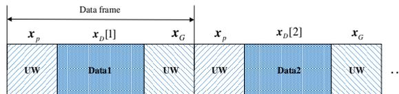
**Fig. 1.** Transmission data frame structure diagram.
