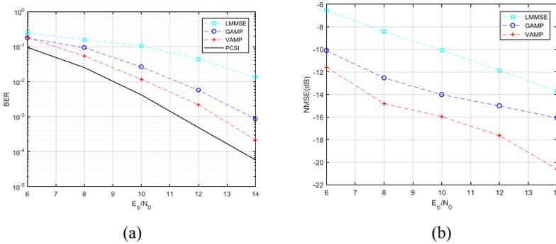
**Fig. 4.** (a) The change curve of BER with  $E_b/N_0$  for different receiving algorithms under UW transmission. (b) The change curve of NMSE with  $E_b/N_0$  for different receiving algorithms under UW transmission.
