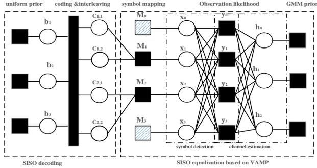
**Fig. 3.** Factor Diagram of SC-FDE System. There are two VAMP full connection subgraphs in the SISO equalizer, virtual box corresponding to symbol detection and channel estimation respectively.
