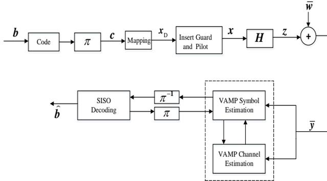
**Fig. 2.** The block diagram of SC block transmission and turbo reception, where  $\pi$  and  $\pi^{-1}$  represent interleaving and deinterleaving, respectively, and  $\mathbf{H}$  represents channel propagation. Virtual frame shows reception using a SISO equalizer that iterates between symbol and channel estimation, which uses VAMP for joint symbol and channel estimation.
