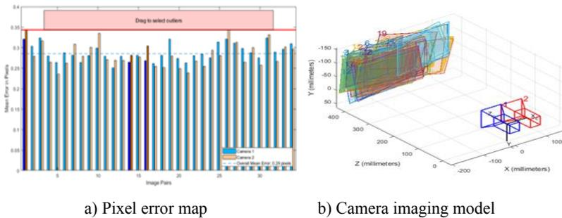
**Fig. 2.** Matlab camera calibration results.
