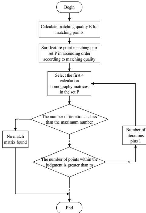
**Fig. 4.** Improved RANSAC algorithm flow char.
