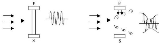
**Fig. 2.** Principle of vortex modulation
