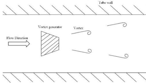
**Fig. 1.** Schematic diagram of Kaman Vortex Street.
