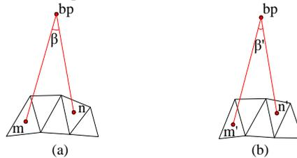
**Fig. 4.** Relative orientation deformation of triangle: (a) the graph before flattening, the directional angle between triangle  $m$  and  $n$  is  $\beta$ , (b) the graph after flattening, the directional angle between triangle  $m'$  and  $n'$  is  $\beta'$ .
