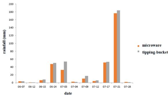
**Fig. 3.** Applicability test of the microwave rain gauge.
