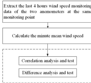
**Fig. 1.** Flow chart of anemometer adaptability test algorithm.
