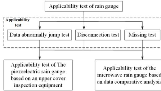
**Fig. 2.** Flow chart of the rain gauges applicability test algorithm.
