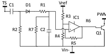
**Fig. 2.** Short circuit protection circuit diagram.
