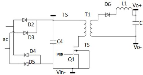
**Fig. 1.** Schematic diagram of switching power supply with flyback topology.
