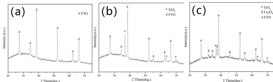
**Fig. 2.** XRD patterns of (a) FTO ,(b) the TiO<sub>2</sub> nanocones and (c) Co<sub>3</sub>O<sub>4</sub>@TiO<sub>2</sub> photoelectrode.
