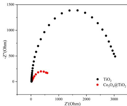
**Fig. 4.** EIS plots for TiO<sub>2</sub> and Co<sub>3</sub>O<sub>4</sub>@TiO<sub>2</sub> photoelectrode.
