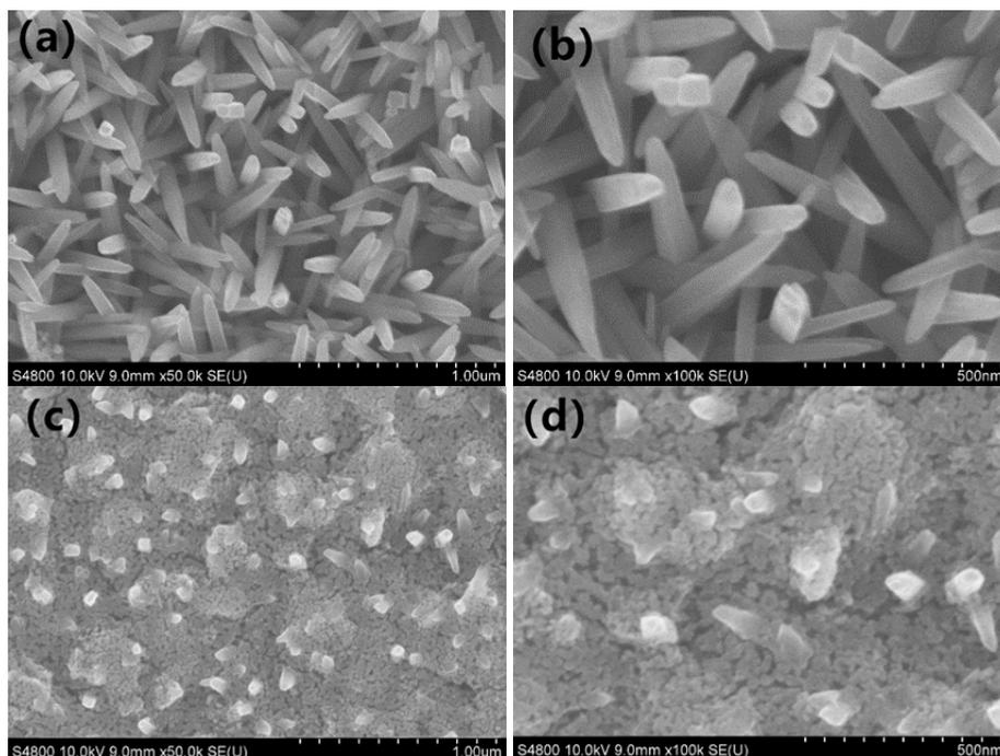
**Fig. 1.** SEM image of (a,b) TiO<sub>2</sub> nanocones, (c,d) Co<sub>3</sub>O<sub>4</sub>@TiO<sub>2</sub> photoelectrode.
