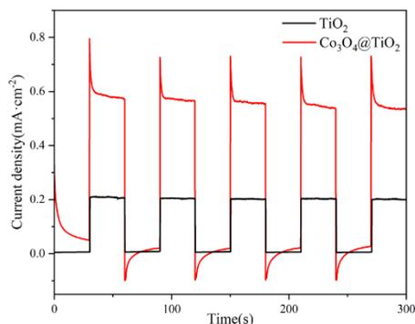
**Fig. 3.** I-t curves of TiO<sub>2</sub> nanocones and Co<sub>3</sub>O<sub>4</sub>@TiO<sub>2</sub> photoelectrode.
