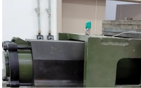
Fig. 6. Acceleration sensor installation.
