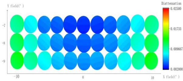
**Fig. 4.** Diattenuation pupil of freeform surface in full field of view.
