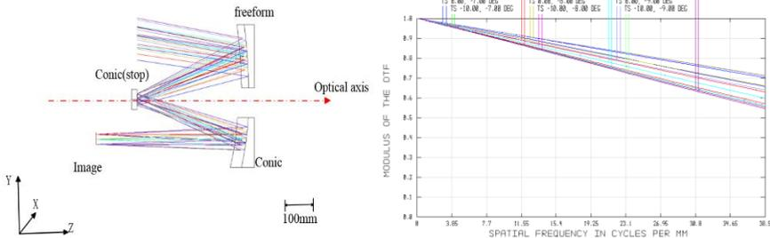
**Fig. 2.** Optical system diagram and MTF diagram.
