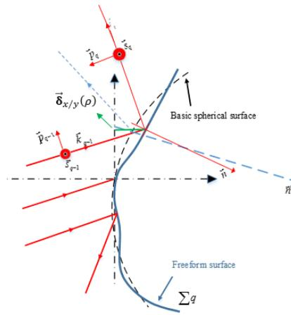
**Fig. 1.** Schematic diagram of polarized light refraction, reflection, and optical path difference on the  $q$ th plane.
