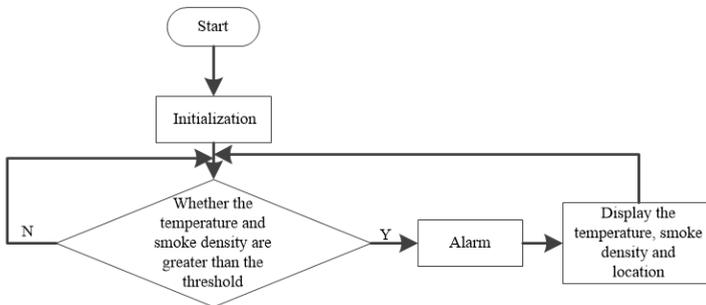
**Fig. 12.** The software flow chart of the display module.
