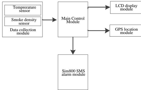
**Fig. 1.** The system block diagram.
