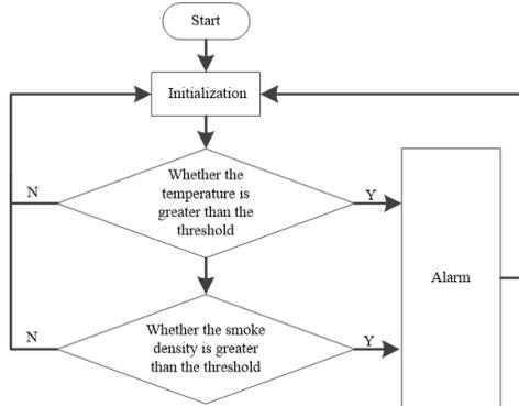
**Fig. 11.** The software flow chart of the alarm module.
