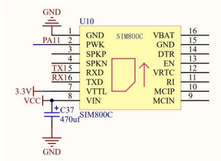
**Fig. 5.** The circuit diagram of Sim800.
