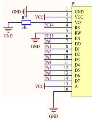
**Fig. 6.** The circuit diagram of LCD1602.
