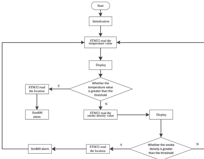
Fig. 8. The software flow chart of the system.
