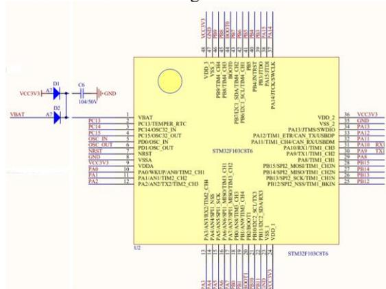
Fig. 2. The pin diagram of STM32F103C8T6.
