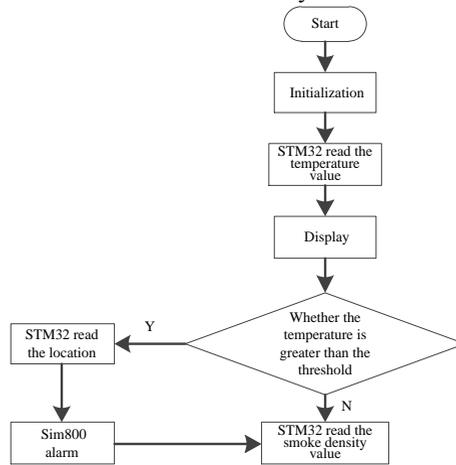
**Fig. 9.** The software flow chart of the temperature monitoring module.
