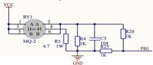
Fig. 4. The circuit diagram of MQ-2 smoke.
