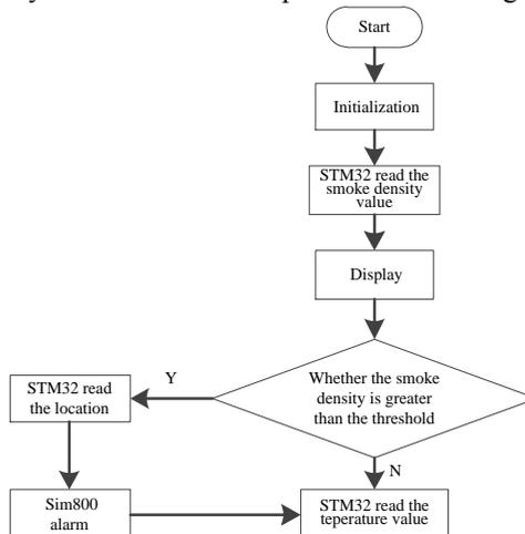
**Fig. 10.** The software flow chart of the smoke density monitoring module.
