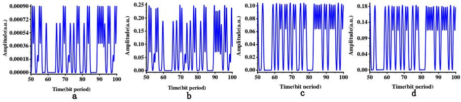
**Fig. 3.** Time-domain waveforms of the downlink 67% duty cycle RZ-4PAM and AMI uplink signals before and after transmission.
