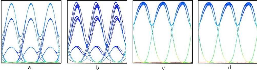
**Fig. 4.** Eye diagrams of the downlink 67% duty cycle RZ-4PAM and AMI uplink signals before and after transmission.
