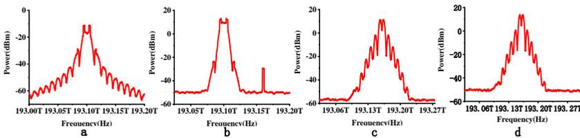
**Fig. 2.** Optical spectrums of the downlink 67% duty cycle RZ-4PAM and AMI uplink signals before and after transmission.
