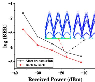
Fig. 5. BER performance of 650nm wavelength.
