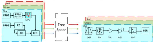
**Fig. 1.** Multi-Color Visible Light Communication System Using 67% RZ-4PAM signals.
