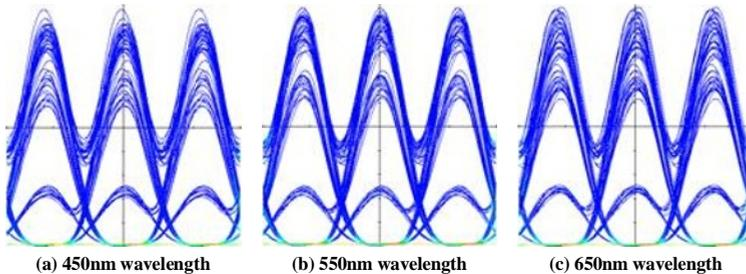
Fig. 4. Eye diagrams measured at different working wavelengths.
