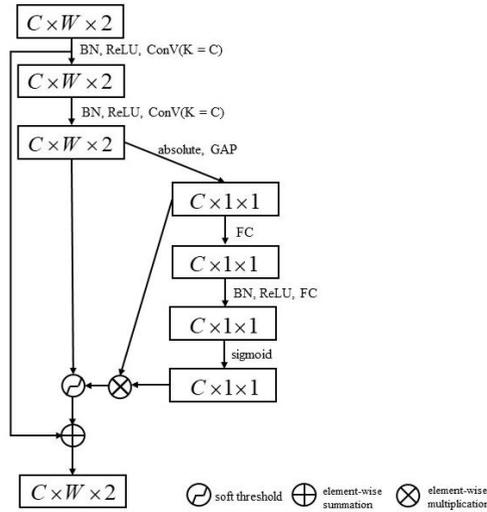
**Fig. 1.** The structure of a residual shrinkage net unit.
