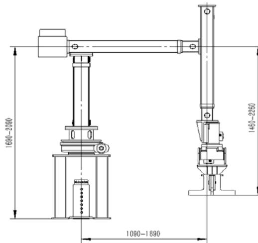
**Fig. 5.** The structural shape of the gripper.
