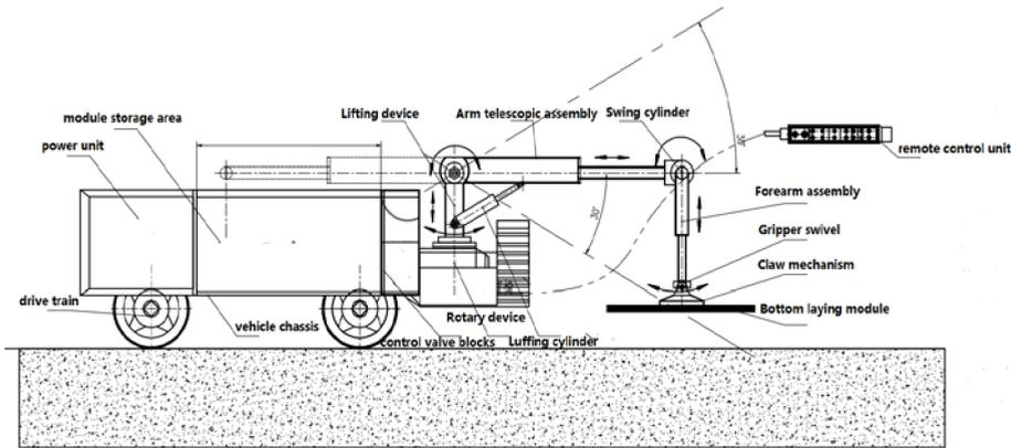
**Fig. 1.** An automatic bottom laying robot.
