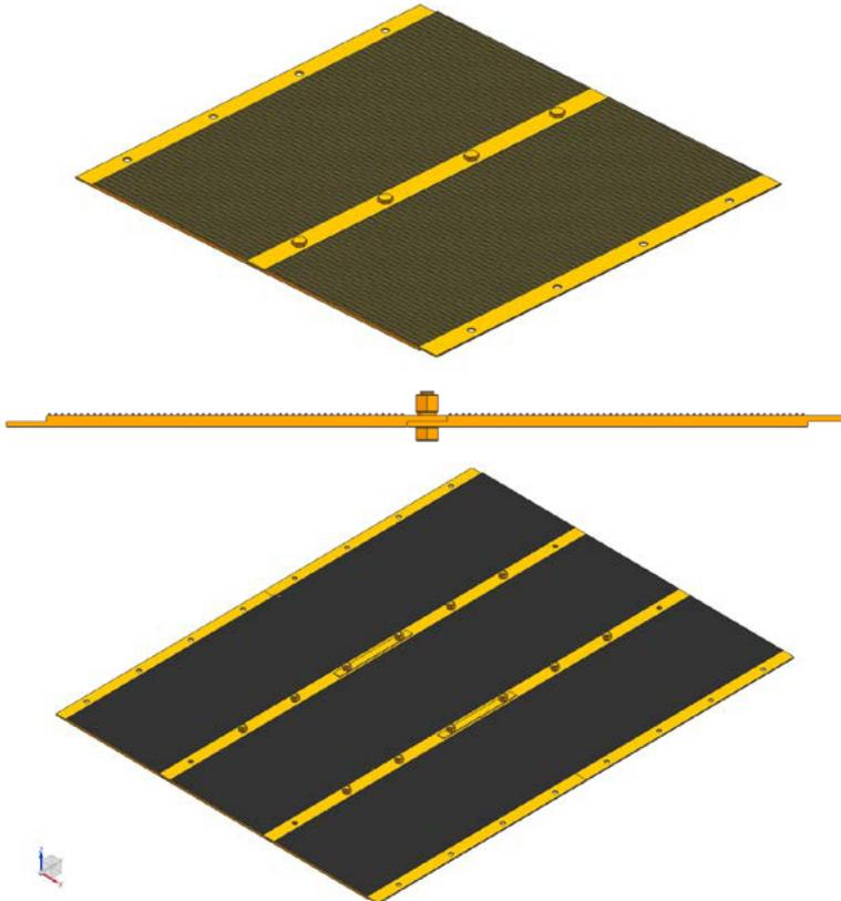
**Fig. 6.** Bottom layer module connection diagram.
