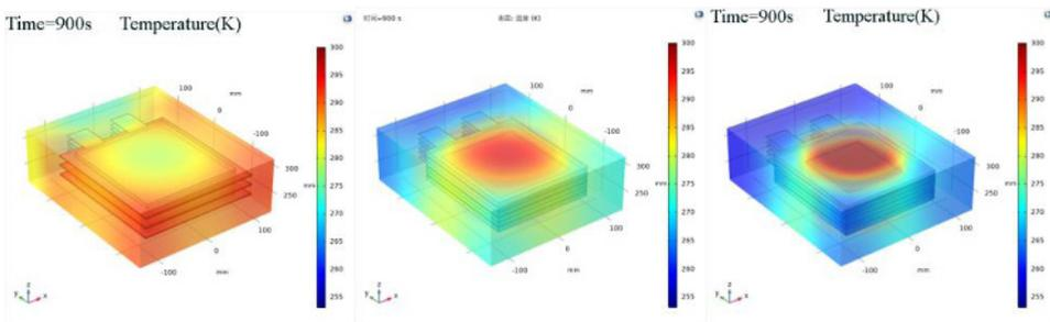
**Fig. 6.** Temperature distribution with different sizes of PTC heating plate at 900 s.
