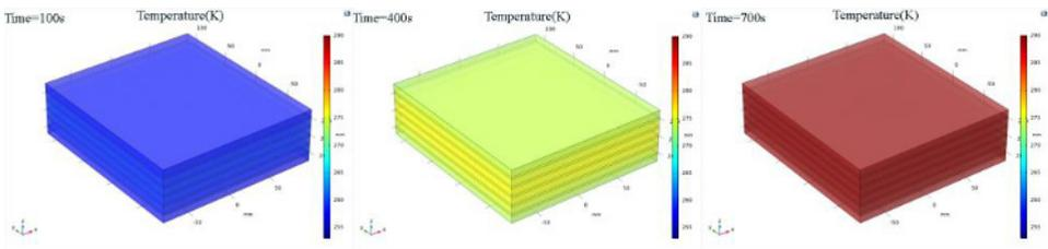
**Fig. 2.** Temperature distribution of PTC preheating scheme at 100 s, 400 s and 700s.
