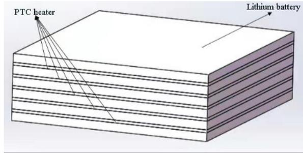
**Fig. 1.** Structure diagram of PTC and lithium battery pack.
