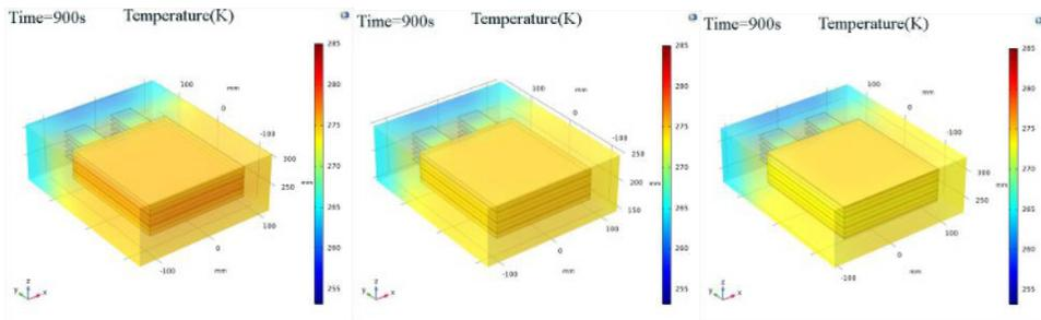
**Fig. 4.** Temperature distribution of lithium battery group combined with two, three, and four PTCs at 900 s.
