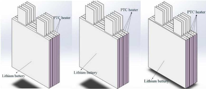
**Fig. 3.** Different combination methods of PTC heating plates and lithium battery.
