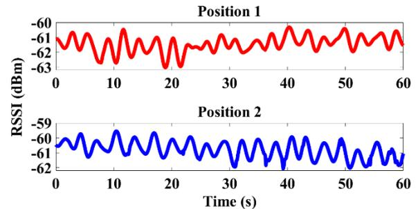
**Fig. 10.** Breathing signals obtained from reading the RFID tag with the 11 mm polyethylene foam and the participant seated.
