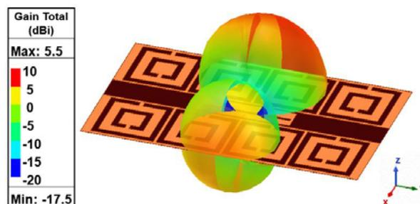
Fig. 4. 3D radiation pattern of the simulated tag.
