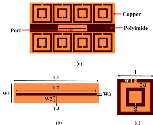
Fig. 1. Simulated RFID tag: (a) tag layers, (b) dimensions of the folded dipole antenna, (c) dimensions of the CSRRs cells.
