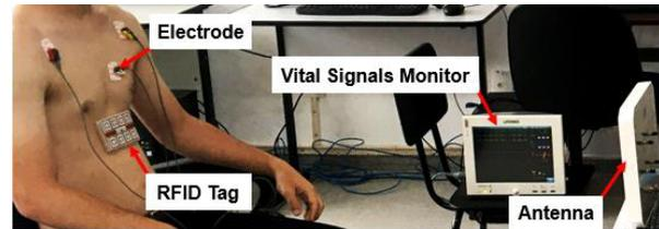
**Fig. 8.** Measurement setting.
