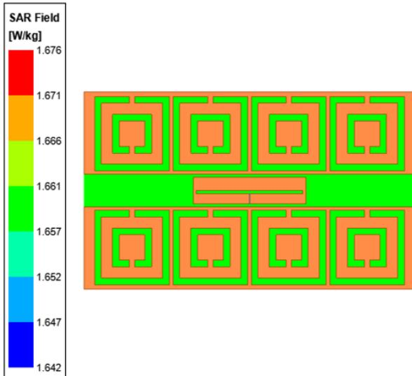
**Fig. 6.** SAR behavior on the RFID tag substrate at the frequency of 915 MHz.
