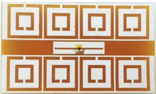
**Fig. 7.** Manufactured RFID tag.
