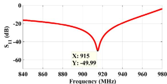
Fig. 2. Reflection coefficient ( $S_{11}$ ) of the simulated tag.
