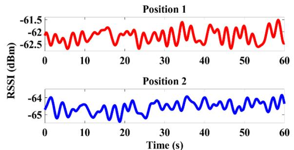
**Fig. 11.** Breathing signals obtained from reading the RFID tag with the 11 mm polyethylene foam and the participant standing.
