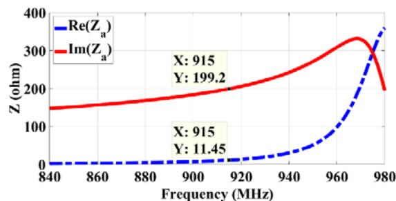
Fig. 3. Input impedance of the simulated tag.
