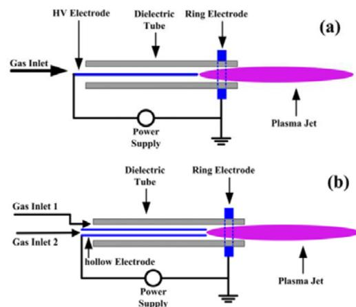
fig 3: Schematic of a DBD-like plasma jet.[5]
