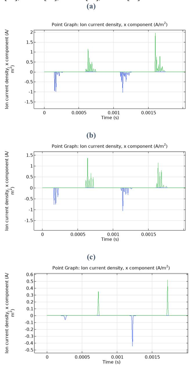
fig 8 : the variation of positive helium ion density, (in blue) next to the dielectric and (in green) next to the cathode with  $f = 1\text{kHz}$  and  $P = 760$  Torr at different discharge distances (a)0.8mm, (b) 1mm and (c)2mm.
