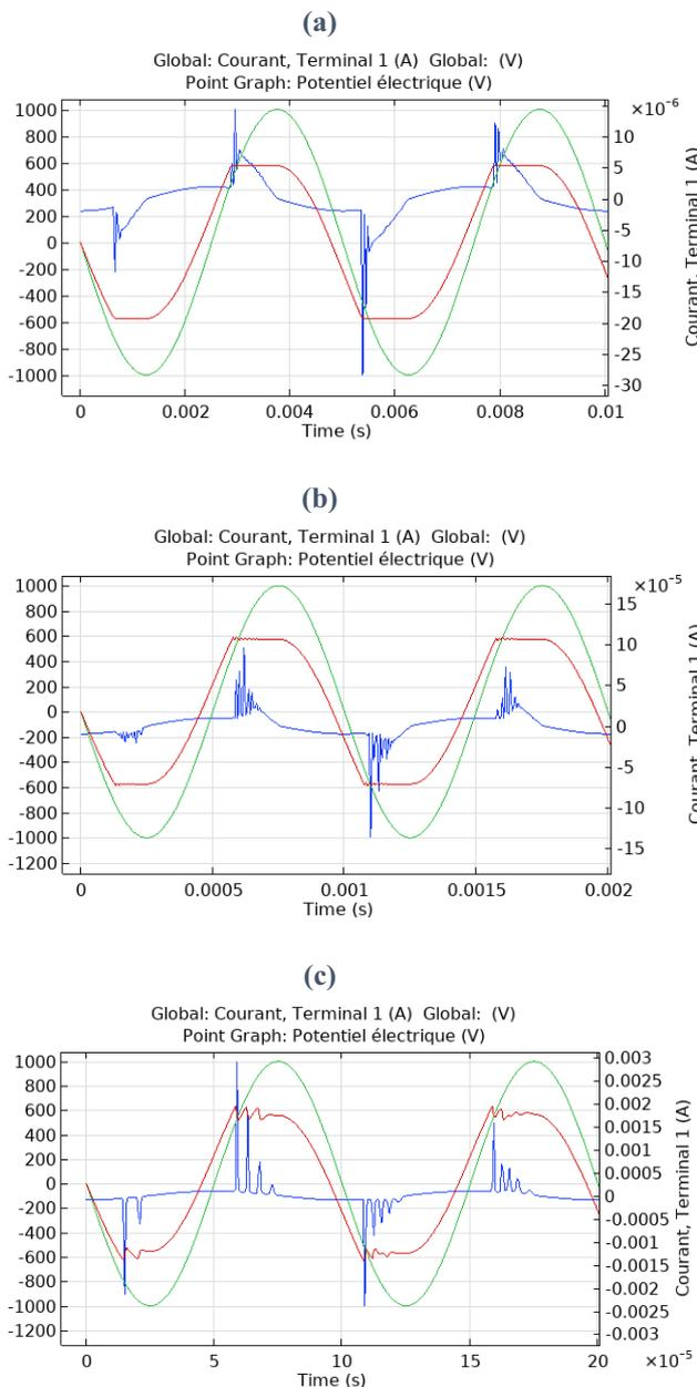
fig 5 : the variation of the breakdown voltage (in red) and of the electric current (in blue) as a function of the applied voltage (in green) with  $d = 0.5$  mm and  $P = 760$  Torr at different frequencies (a) 200Hz, (b) 1kHz and (c) 10kHz.
