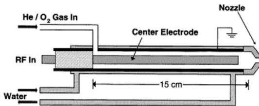
fig 1: Schematic of the dielectric-free electrode atmospheric-pressure plasma jet[11]
