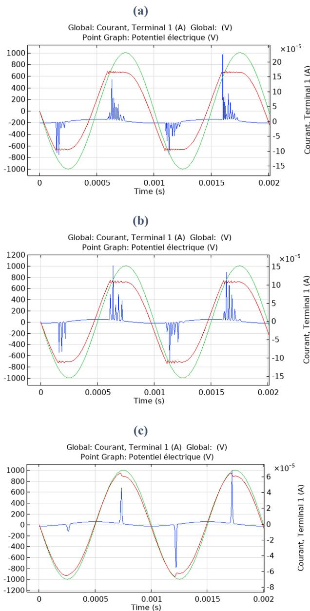
fig 7 : the variation of the breakdown voltage (in red) and of the electric current (in blue) as a function of the applied voltage (in green) with  $f = 1\text{kHz}$  and  $P = 760$  Torr at different discharge distances (a)0.8mm, (b) 1mm and (c)2mm.
