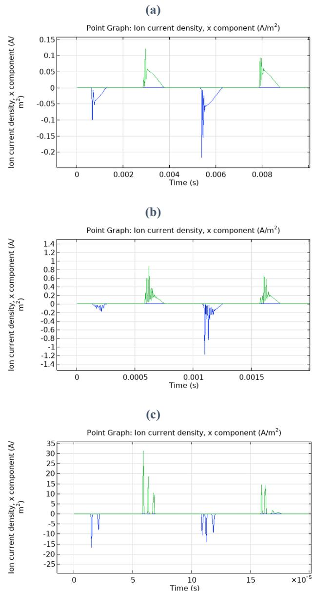
fig 6 : the variation of positive helium ion density, (in blue) next to the dielectric and (in green) next to the cathode with  $d = 0.5$  mm and  $P = 760$  Torr at different frequencies (a) 200Hz, (b) 1kHz and (c) 10kHz.
