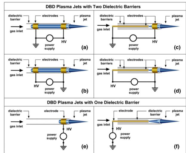
fig 2 : Different configurations of DBD plasma jet [13]
