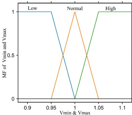
**Fig. 6.** Inputs membership functions of the fuzzy logic controller.
