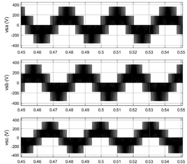
Fig. 5. Stator voltages of induction motor
