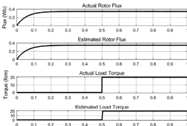
Fig. 3. Estimated rotor flux and load torque
