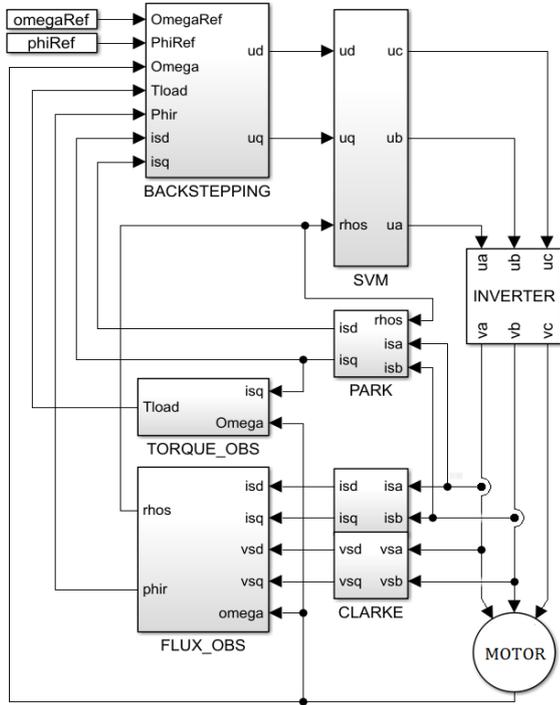
Fig. 1. Synoptic diagram of Backstepping control
