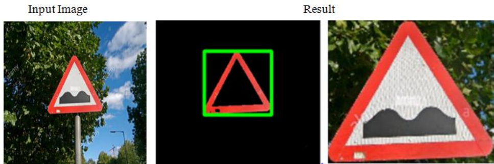
Fig. 15. ROI created and detecting red colour object.
