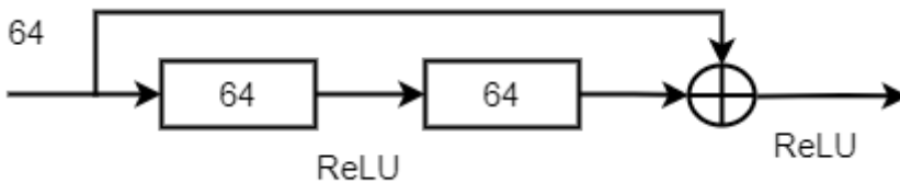
Figure 4. A residual block in a ResNet model. The map dimension can be 64, 128, 256, or 512
