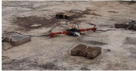
Fig. 31. Tied flight test of quadcopter.
