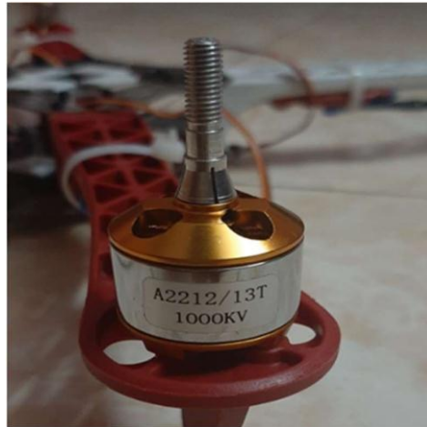
Fig. 6. Brushless DC motor used for propulsion system.
