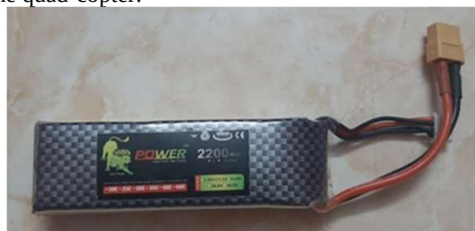
Fig. 8. Lithium Polymer battery (2200mAh).
