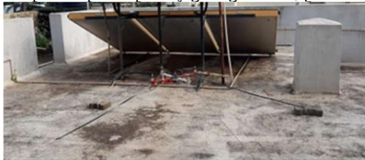
Fig. 32. Tied Quadcopter flight with maximum throttle.
