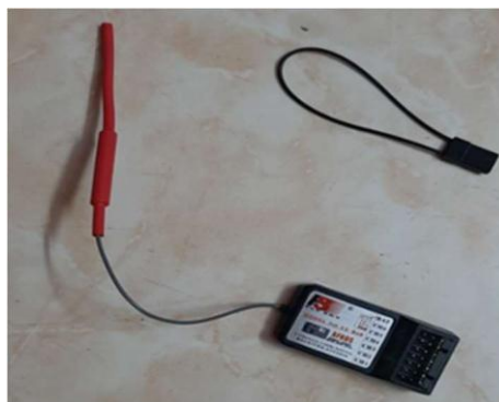
Fig. 14. Radio receiver and binding cable.
