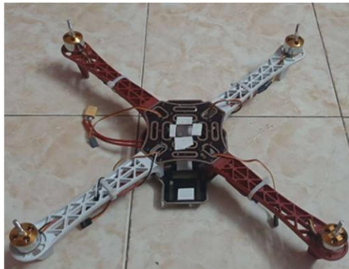
Fig. 5. Glass fibre frame of the developed quadcopter.
