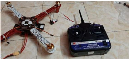
Fig. 23. Binding of transmitter and receiver.
