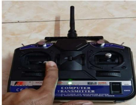
Fig. 27. Arming the quadcopter by transmitter.
