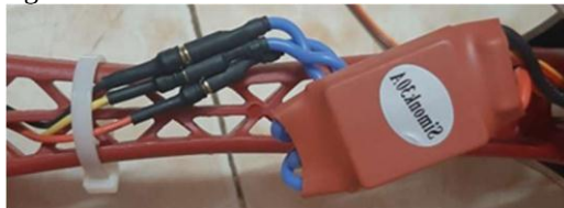
Fig. 12. Electronic speed controller of 30A.
