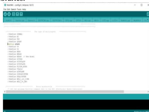
Fig. 16. Configuration of Multicopter type in Arduino IDE.
