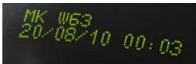
Fig. 8. Restored image of the drip-jet marking.
