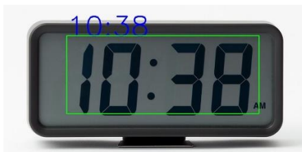
Fig.3. Example of text recognition result using PARSeq model.
