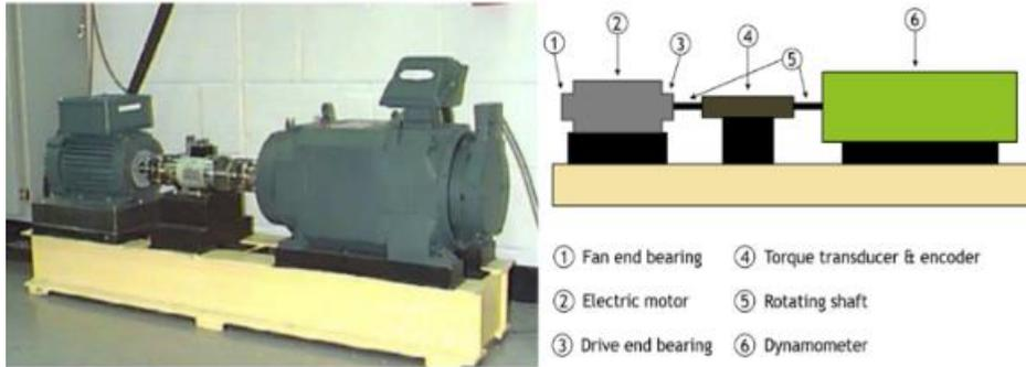
Fig. 2. The CRWU bearing datasets used in this paper.
