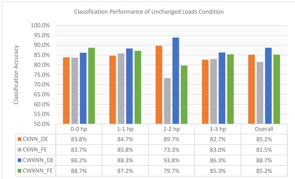
**Fig. 3.** The classification performance of CKNN and CWKNN of unchanged loads condition
