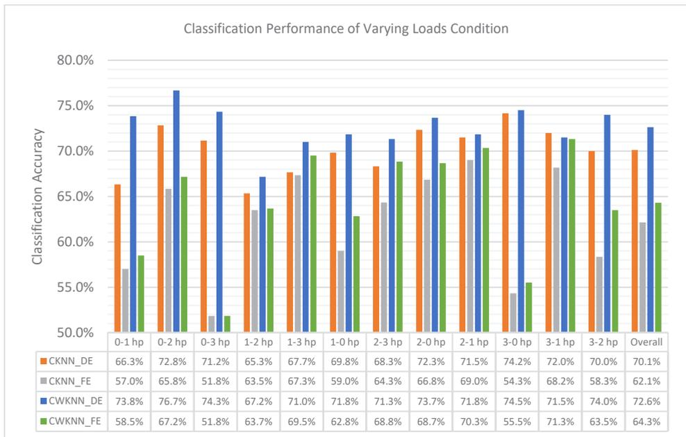
**Fig. 4.** The classification performance of CKNN and SWKNN of varying loads condition.
