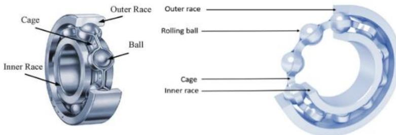
Fig. 1. The elements of bearing: Outer Race, Inner Race, Cage and Ball [3], [4]
