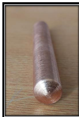
Fig 4 Convex shape copper electrode
