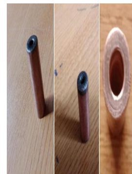
Fig 5 Hollow shape copper electrode
