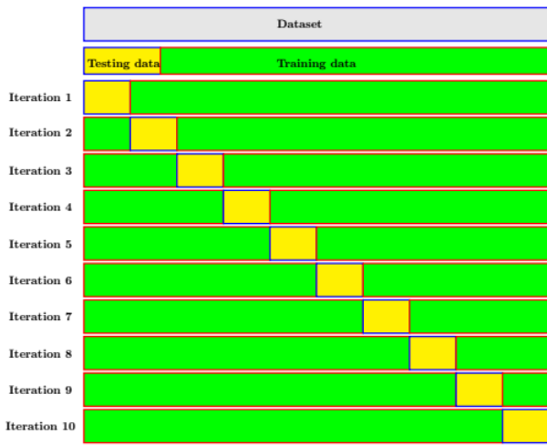
Figure 4. Example of dataset divided using the 10-fold cross-validation method
