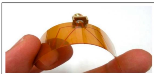
Fig. 3. Fabricated prototype of the pattern-reconfigurable antenna on flexible polyimide.
