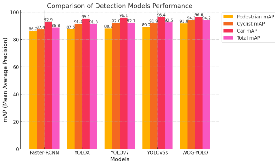
Fig. 1 Comparison of the performance of different OD models (Faster-RCNN, YOLOX, YOLOv7, YOLOv5s, and WOG-YOLO) based on mAP scores for pedestrian, cyclist, and car detection (Picture credit: Original).
