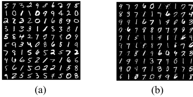
Fig. 5. Comparison of real images of the test dataset for GAN and images generated by GAN model training. (a) real image, (b) generated image (Photo/Picture credit: Original).
