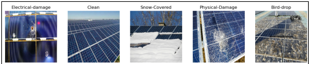
Figure 5: Identification of Defects in Solar Panels
