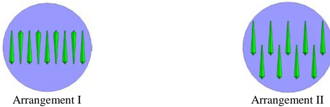
Fig. 5. The arrangement of the okra in the turntable for microwave drying (a) Arrangement I, and (b) Arrangement II.
