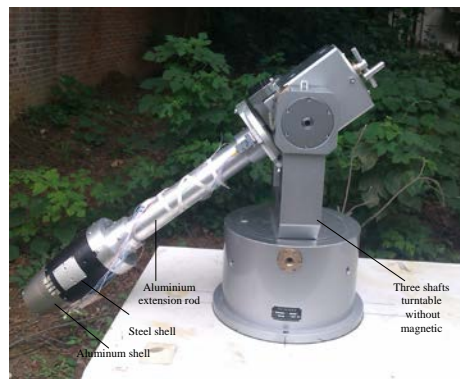
Fig. 2. The axis turntable to install extension bar and missile body.
