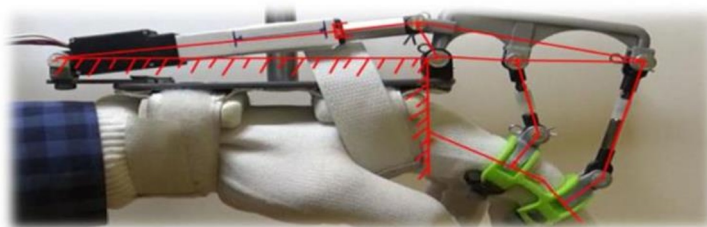
Fig. 2. Traditional RobHand conFiguration with a single finger [10]
