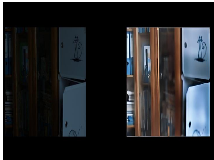
Fig. 1. Qualitative comparison: (Left) low-light input image, (Right) ASPG-MSLIE enhanced output. Natural colours are restored by the model, reconstructs delicate features like wood grain and cat illustration, and removes a substantial amount of noise, with no loss of structural boundaries.
